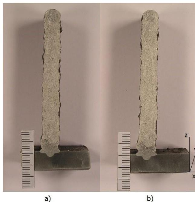
**Fig. 6: Macrostructures of the end (a) and the middle of the wall (b)**
