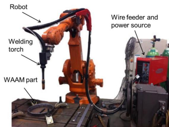
Fig. 1: Example of WAAM system (right) [6]
