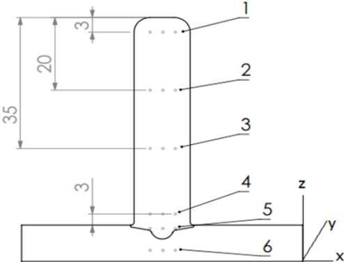
**Fig. 8: Points for microhardness measuring**
