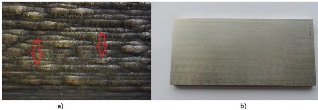
**Fig. 4: Pores on lateral sides (a); deposited wall after milling (b)**
