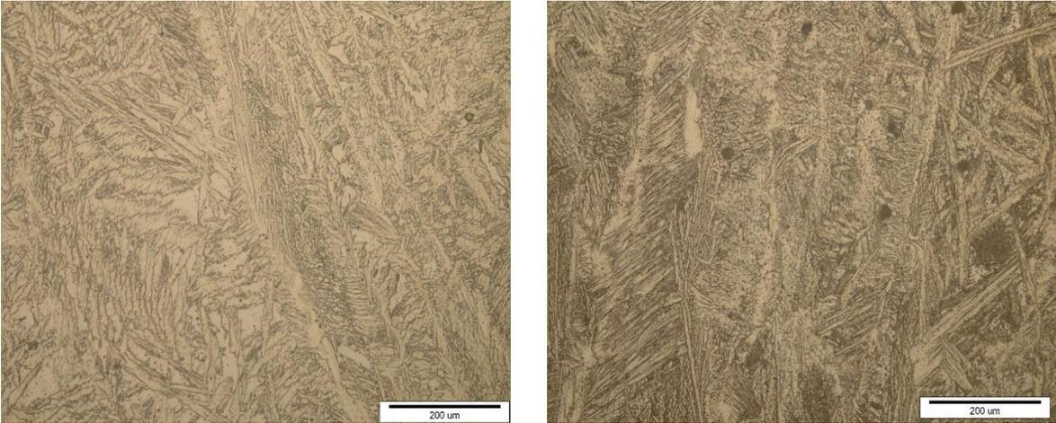
**Fig. 7: Microstructure of the deposited wall**
