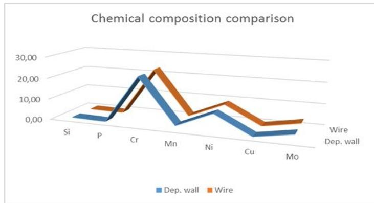
**Fig. 5: Chemical composition comparison between the deposited wall and the wire**
