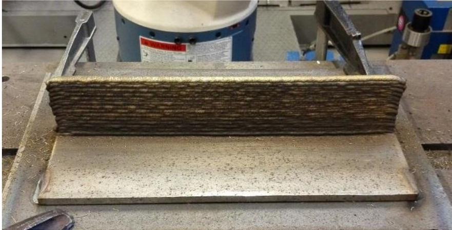
**Fig. 3: Deposited WAAM wall**
