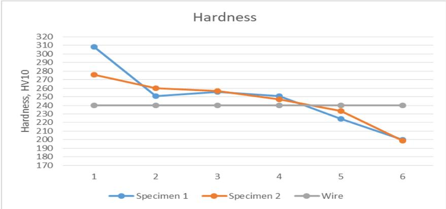
**Fig. 8: Hardness profiles for both specimens compared**
